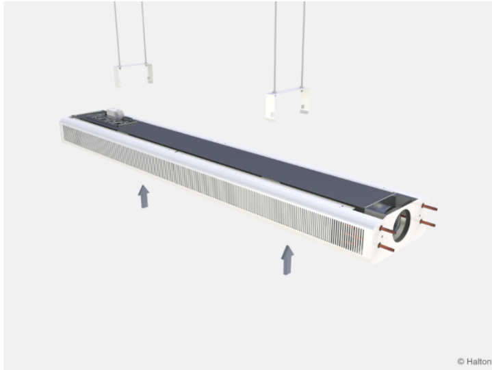
Fig. 26. Fixing of the beams done by pushing the beam to the ceiling brackets.
